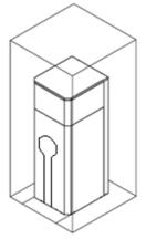
When placing the appliance be aware that a minimum clearance of 24" (60cm) must be provided at the front to allow easy access to the heat exchanger.
