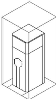
When placing the appliance be aware that a minimum clearance of 24" (60cm) must be provided at the front to allow easy access to the heat exchanger.
