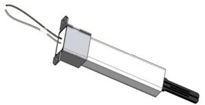
During trial for ignition a properly operating igniter will generate 3.2+/-0.2A which is above the flame signal required by the ignition module for reliable and consistent operation. It is recommended that the hot surface igniter be replaced every 4,000 hours of appliance operation to maintain peak ignition efficiency.
