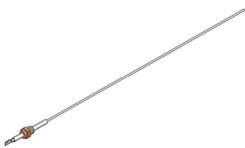
The ignition module relies on the flame sensor to provide a flame rectification signal. Oxide deposits, improper placement or damaged ceramic insulator will result in insufficient signal leading to ignition module lock out. For proper operation minimum 0.2 Vdc must be fed back to the module. Oxide deposit on the sensor rod must be removed with steel-wool. Do not use sand-paper since this will contaminate the surface.
