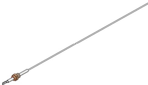
The ignition module relies on the flame sensor to provide a flame rectification signal. Oxide deposits, improper placement or damaged ceramic insulator will result in insufficient signal leading to ignition module lock out. For proper operation minimum 0.2 Vdc must be fed back to the module. Oxide deposit on the sensor rod must be removed with steel-wool. Do not use sand-paper since this will contaminate the surface.
