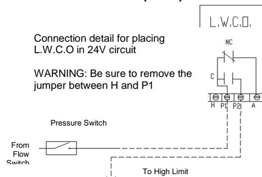
**Figure 18: Low Water Cut Off Electrical Connections (ITT)**
