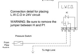
Figure 18: Low Water Cut Off Electrical Connections (ITT)
