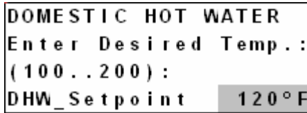
Figure 70: Domestic Hot Water Setpoint
