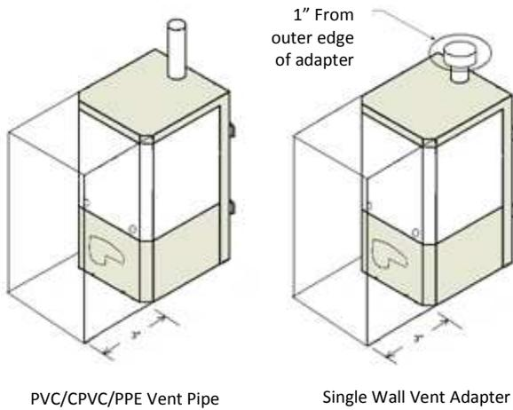
**Figure 2: Floor Mount Clearance from Combustibles**
