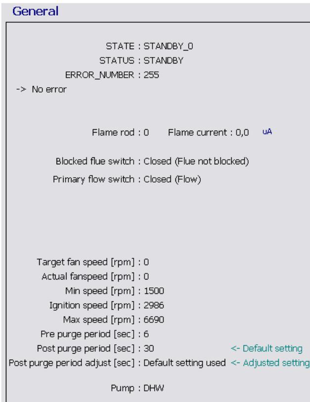
To change a blue coloured parameter, place the cursor over a parameter and double-click. This will bring up a window to enter the desired values of operation. Take note of the minimum and maximum values that can be entered, as the values entered MUST be within this range
