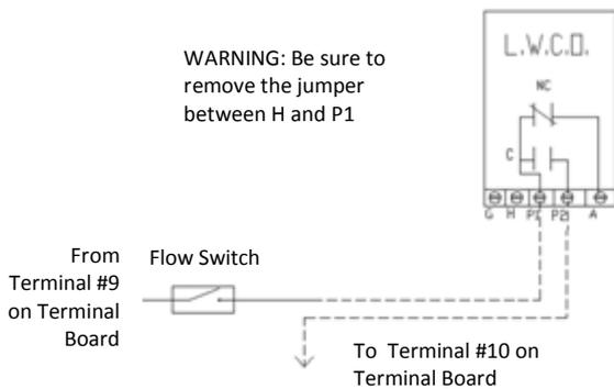
**Figure 21: Low Water Cut Off Electrical Connections (ITT)**
