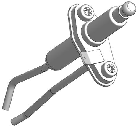
During a trial for ignition sequence a properly operating igniter will generate a continuous spark with a 9/64" (3.6mm) spark gap. It is recommended to clean the direct spark igniter using steel wool as required. **DO NOT** use sandpaper or grit-cloth since this will contaminate the metal surface.
