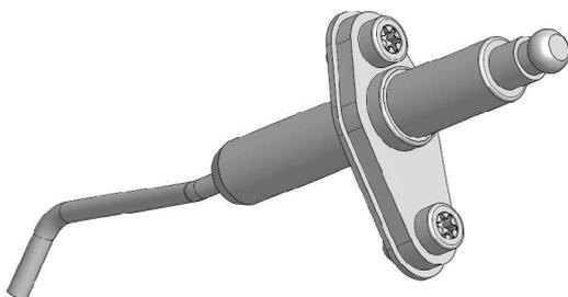
The ignition module relies on the flame sensor to provide a flame rectification signal. Oxide deposits, improper placement or damaged ceramic insulator will result in insufficient signal leading to ignition module lock out. For proper operation minimum 1.25  $\mu$ A DC must be fed back to the module. Oxide deposit on the sensor rod must be removed with steel-wool. **DO NOT** use sand-paper or grit-cloth since this will contaminate the metal surface.
