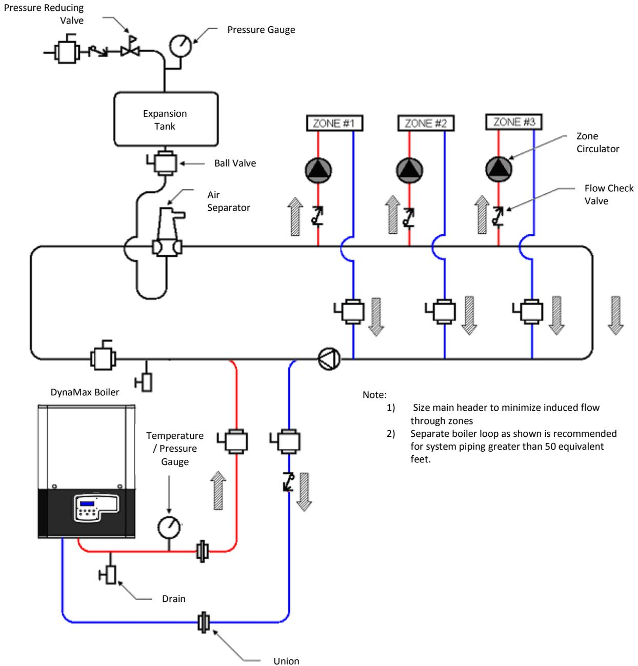
**Figure 70: Single Combination Boiler Zoned Piping Arrangement**
