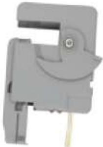
The flow proving device is designed to detect when flow is present. This is done by detecting the amount of current (amperes) that exists in the neutral wire from the pump. When the current becomes too low a flow switch error is displayed indicating a lack of water inside the boiler. The flow proving device is provided on all DynaMax wall mount models (DM 80 – 250) and combination floor model units (213 – 803). This switch is factory wired.
