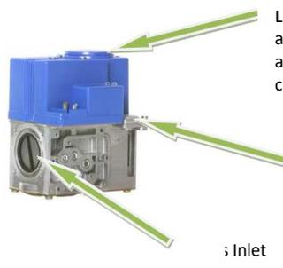
Lift top cover to access high fire air/gas ratio adjustment (use 3mm allen key for adjustment, counter-clockwise increases CO<sub>2</sub>)
