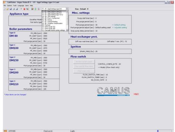
To adjust ignition fan speeds. Use the pull down menu or the function keys on the keyboard, select Settings. This will bring up the Settings screen.
