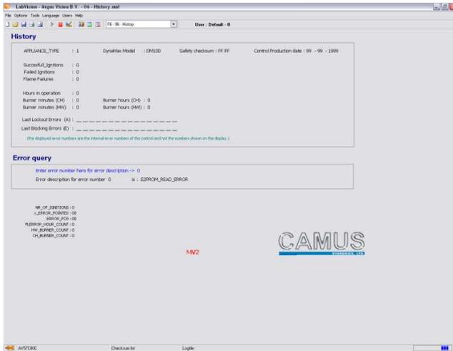
The blocking and lockout errors are separated into their own respective rows and are identified by their respective error codes. This assists with diagnostic and service work as the behaviour of the boiler can be tracked.
