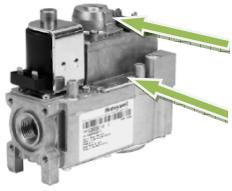
High fire adjustment, (use 3mm allen key for adjustment, counter-clockwise increases CO<sub>2</sub>)
