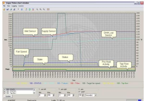
To select the parameters that need to be viewed or recorded, a Parameter Selection Box on the bottom left-side of the screen contains all the parameters that LabView can track. To view or record the parameter that is required, click the check box beside each parameter. When finished selecting the parameters required, click on Update and this will refresh the logging screen.
