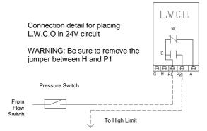
Figure 20: Low Water Cut Off Electrical Connections (ITT)
