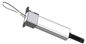
During trial for ignition a properly operating igniter will generate a minimum 3.2+/-0.2A which is the current required for reliable ignition. It is recommended that the hot surface igniter be replaced every 4,000 hours of appliance operation to maintain peak ignition efficiency.
