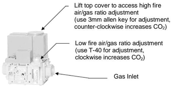
Lift top cover to access high fire air/gas ratio adjustment (use 3mm allen key for adjustment, counter-clockwise increases CO<sub>2</sub>)
