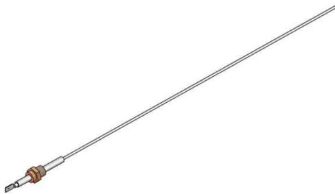
The ignition module relies on the flame sensor to provide a flame rectification signal. Oxide deposits, improper placement or damaged ceramic insulator will result in insufficient signal leading to ignition module lock out. For proper operation minimum 0.8 Vdc must be fed back to the module. Oxide deposit on the sensor rod must be removed with steel-wool. Do not use sand-paper since this will contaminate the surface.
