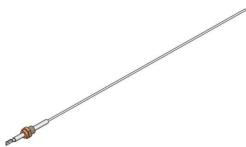
The ignition module relies on the flame sensor to provide a flame rectification signal. Oxide deposits, improper placement or damaged ceramic insulator will result in insufficient signal leading to ignition module lock out. For proper operation minimum 0.8 Vdc must be fed back to the module. Oxide deposit on the sensor rod must be removed with steel-wool. Do not use sand-paper since this will contaminate the surface.
