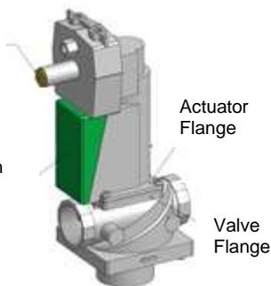
**Figure 11: DR3500 – 5000 SKP25 Regulating Gas Valve Actuator & SSOV**
