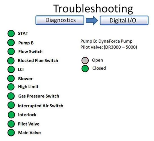
Flow Switch = Flow Switch, Low water cutoff (if equipped), Water Pressure Switch (30 PSI)
