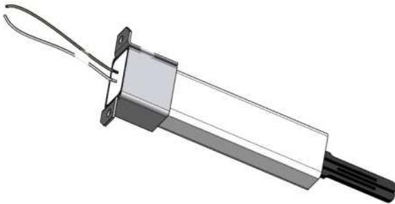
During trial for ignition a properly operating igniter will generate a minimum  $3.2 \pm 0.2A$  which is the current required for reliable ignition. It is recommended that the hot surface igniter be replaced every 4,000 hours of appliance operation to maintain peak ignition efficiency.
