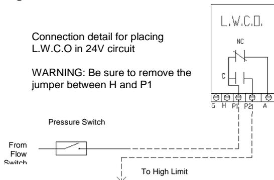
**Figure 20: Low Water Cut Off Electrical Connections (ITT)**
