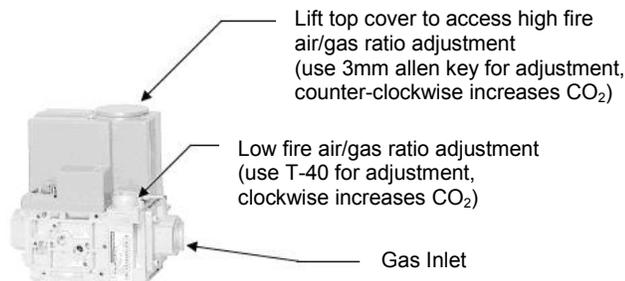
Figure 10: AV800 – 4000: 1:1 Air/Gas Ratio Control Valve
