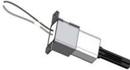
During trial for ignition a properly operating igniter will generate  $3.2 \pm 0.2A$  which is above the current required for reliable ignition. It is recommended that the hot surface igniter be replaced every 4,000 hours of appliance operation to maintain peak ignition efficiency.
