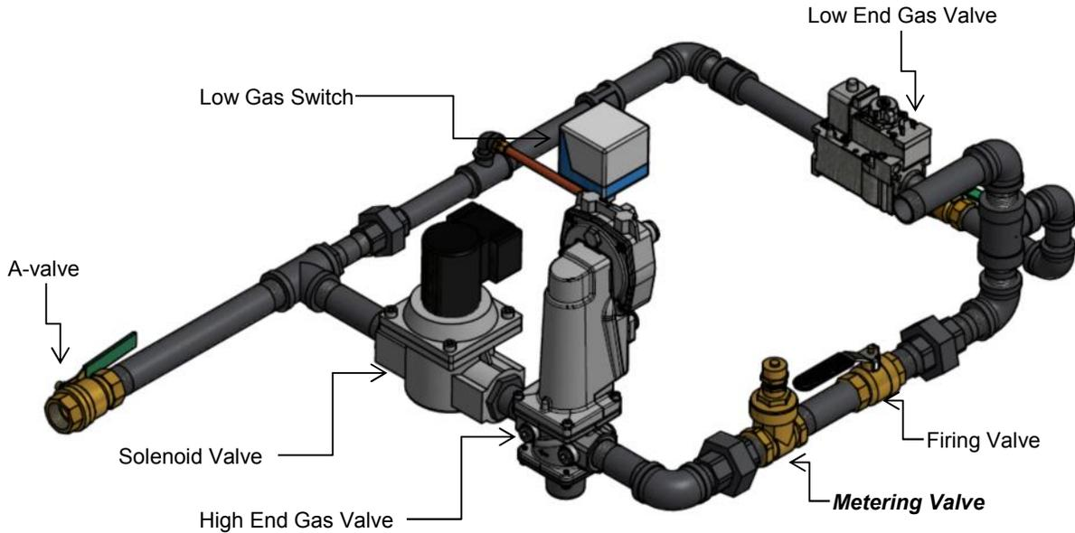
Figure 39: Typical Gas Train (Models AV2500-3000)
