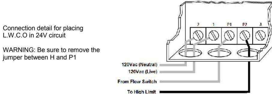
Figure 21: Low Water Cut Off Electrical Connections (ITT)
