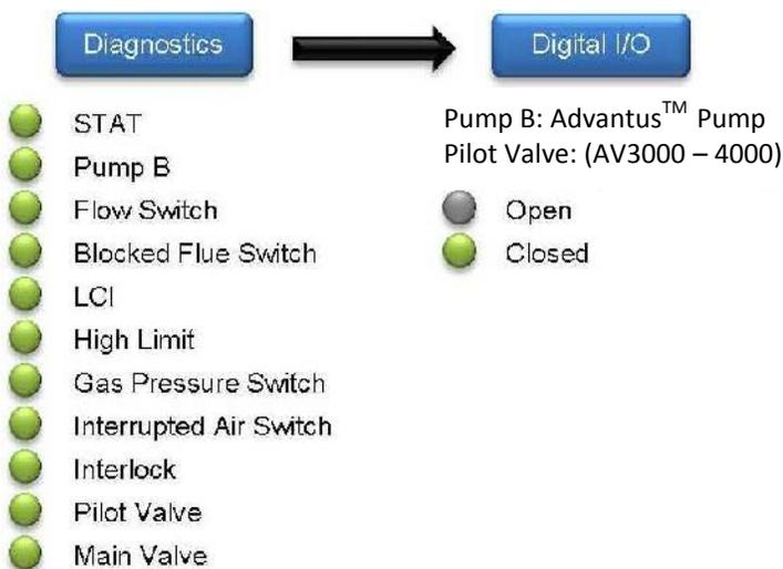
**Flow Switch** = Flow Switch, Water Pressure Switch (30 PSIG), Low Water Cut Off (if equipped)
