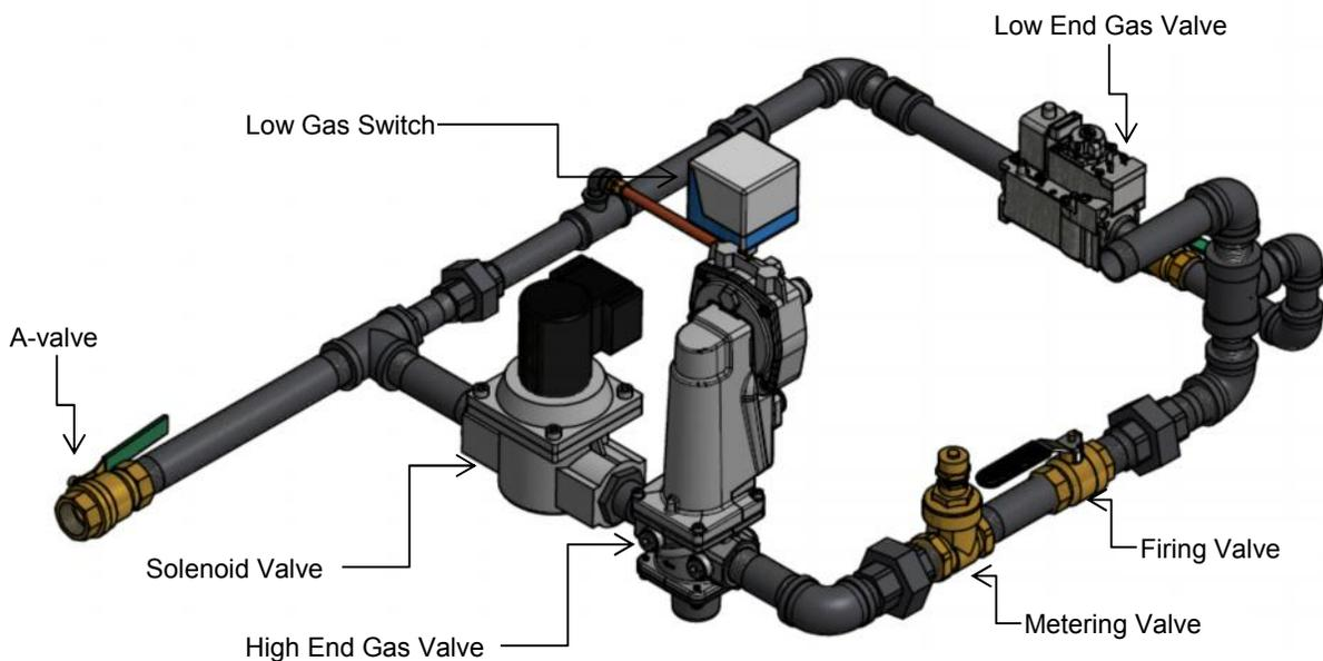
Figure 14: Typical Gas Train (Models AV2500-3000)
