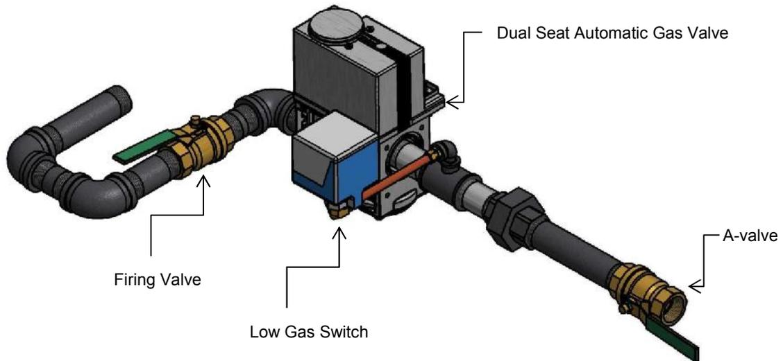
Figure 13: Typical Gas Train (Models AV800 -2000)
