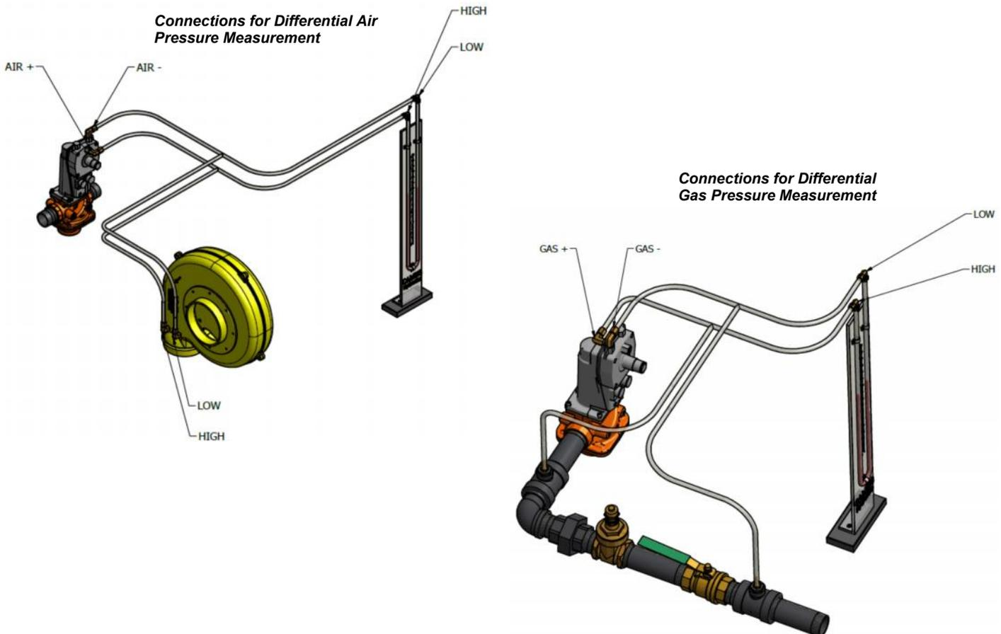
The 1:1 air/gas ratio control actuator has embossed markings identifying + air, - air, + gas & - gas connections. Using a test hose assembly fitted with tees, connections can be made from the manometer to the appropriate ports on the actuator.
