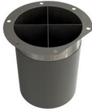
This appliance uses a single cylindrical burner installed vertically into the combustion chamber at the top of the heat exchanger. The burner consists of a round mounting flange welded to a mixing tube. The flange provides the transition from the combustion air fan into the burner. The mixing tube is covered with a knitted alloy material that forms the burner port surface. The burner port surface can sustain operation from a blue flame down to infrared conditions as the burner input varies.
