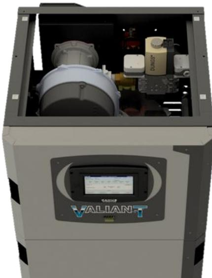
The Valiant FT Series II does not necessarily require access through the sides and can be placed adjacent to each other with minimum clearances. However, it is highly recommended to allow for at least a minimum clearance of 10" on the appliance's right-hand side. This allows for easy access to maintain the combustion air filter. Access panels from the sides of the unit are also provided to make the
