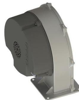
The Valiant FT Series II uses a modulating air fan to provide combustible air/gas mix to the burner and push the products of combustion through the heat exchanger and venting system. The fan assembly consists of a sealed housing and fan wheel constructed from spark resistant cast aluminum. The fan is operated by a fully enclosed 120 VAC, Single-Phase EC/DC electric motor. The fan housing and motor assembly is fully sealed and SHOULD NOT be field serviced.
